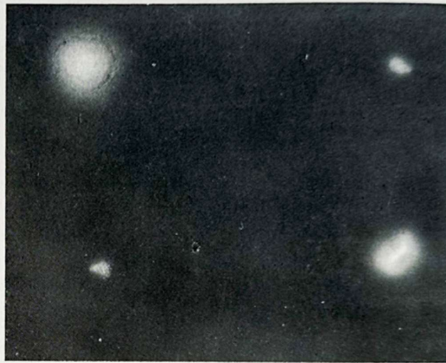
FIG. 21.—Photograph of crystals of fluor-spar after exposure to radium radiations.
