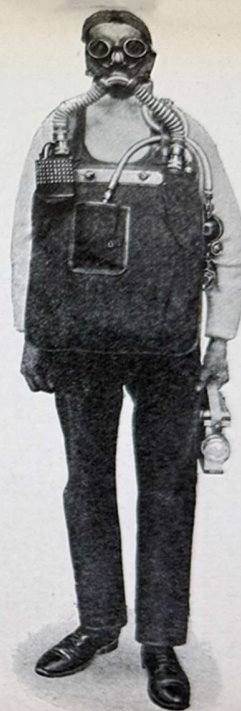
Fig. XXIV.—Front view of the "Proto" apparatus. Mouth-piece and nose-clip type. Showing breathing-tubes and breathing-bag.
