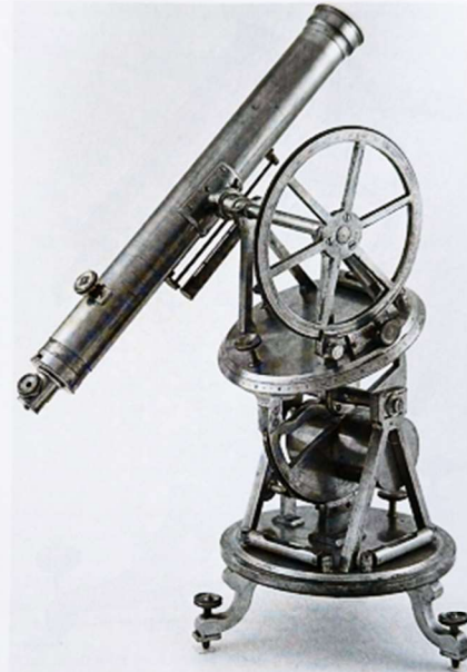
7.18 A universal equatorial mounting and telescope, signed 'Adams, London', with a long declination axis and circular declination scale, similar to the design depicted in figure 7.17. The diameter of the base is 7 inches, a size commonly used by the Adams firm for Ordnance theodolites. ( Private collection ) Earlier equatorial mountings by George Adams, based on the rather less stable mid-eighteenth century design by James Short, are located at the University of Bologna (formerly the property of Lord George Cowper), and the Harvard Collection, Massachusetts (acquired second-hand in 1803; see Wheatland, Apparatus of Science pp. 27–9).
